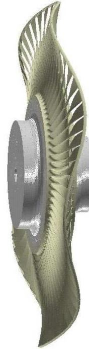
**FIGURE 11.** TURBINE BLADE MODE SHAPE FOR NODAL DIAMETER 5
